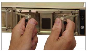
Figure 1 | Pluggable canisters are easy to insert and remove.
