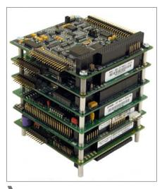
Figure 2 | PC/104 stackable embedded
