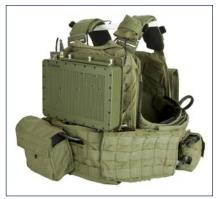
Figure 1 | The Wearable Computer System from Crystal Group weighs less than 10 pounds.
